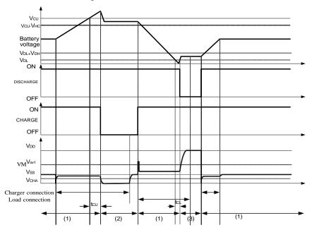
Figure 5-1 Overcharge and Overdischarge Voltage Detection
