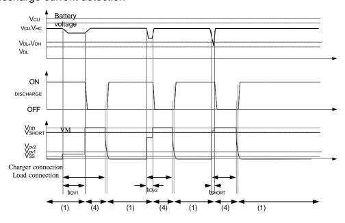
**Figure5-2 Overdischarge Current Detection**
