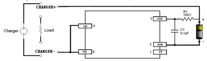
Fig 6 XB5352G in a Typical Battery Protection Circuit
