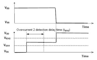
Figure 4. Overcurrent delay time
